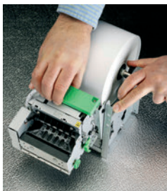
Easy Paper Load – simply “lift and tilt” mechanism and insert paper
